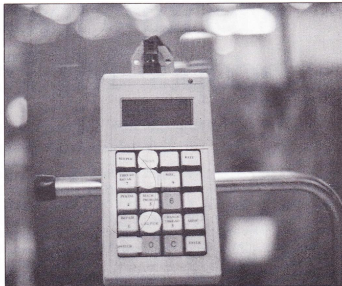
Picture above shows team system working at Meritina, using Mr Engineer. Below, the Mr Engineer operator keyboard providing the following features: Name. Rate for Job. Expected Performance. Stitches Sewn on Garment. Actual Efficiency. Cycle Countdown. Red Pacing Light.
