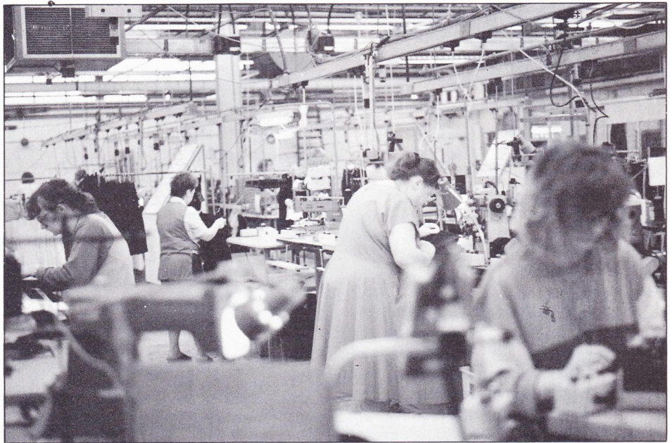
Picture above shows team system working at Meritina, using Mr Engineer. Below, the Mr Engineer operator keyboard providing the following features: Name. Rate for Job. Expected Performance. Stitches Sewn on Garment. Actual Efficiency. Cycle Countdown. Red Pacing Light.
